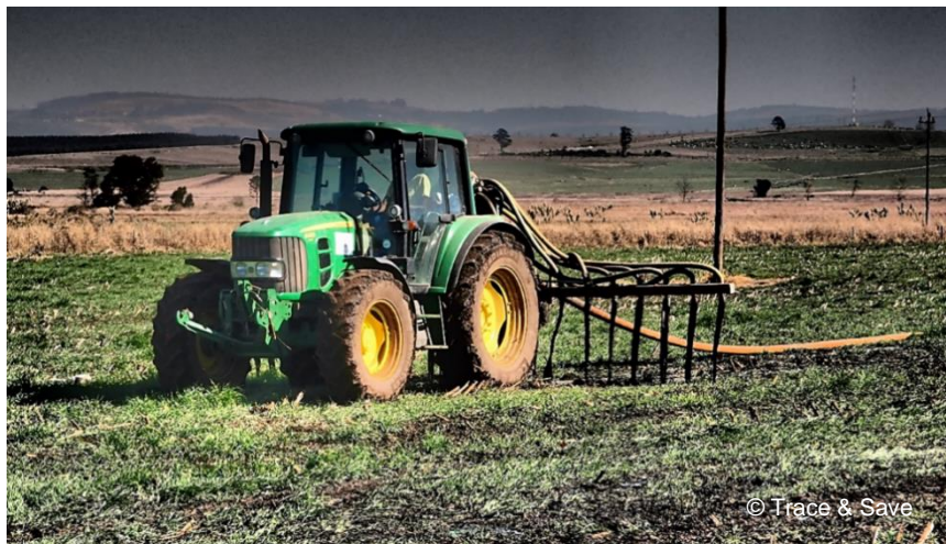
An effluent spreader is used for the effective use of dairy effluent on pastures and improved soil fertility.
