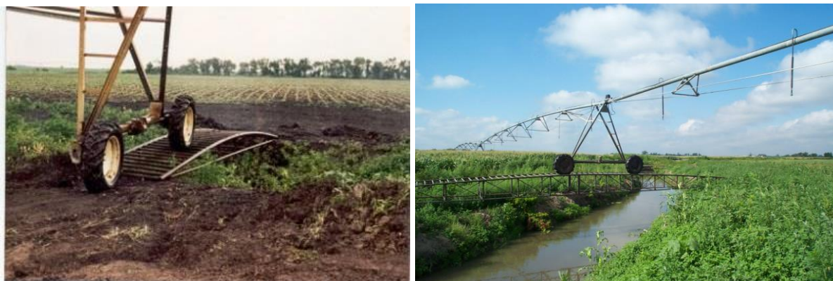
Figure 13. Examples of welded steel pivot crossings over streams and rivers (Commercial suppliers).
